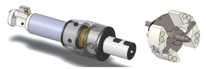
The new **centrifugal force actuated** Autofacers can be used for automatic backspot facing whereever flywheel or bump style actuation is not possible. The cutter blade will automatically open at a pre-determined rpm. The Autofacer consisting of actuation modul and
