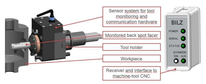
AUTOFACER reverse countersinks are used whenever the surface to be machined is only accesible through a bore, e.g. within a housing. The cutter blade will be opened by changing the sense of rotation when the tool is in working position.
