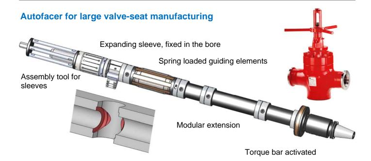
Slide valves made from INCONEL 718 can be machined fast and safely on a machining centre without U-axis. The tool length can be easily adjusted with extensions due to the modular design. Expanding sleeves will compensate bore diameters variations and will thus safely guide the tool.
